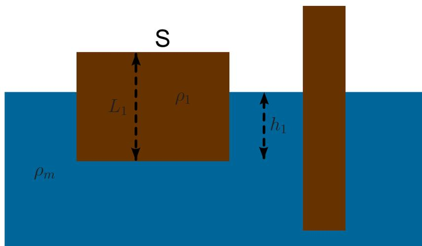
$$\text{a) } S L_1 \rho_1 = S h_1 \rho_m \quad h_1 = L_1 \frac{\rho_1}{\rho_m} = 32 \times \frac{2.9}{3.3} = 28.12 \text{ km}$$
